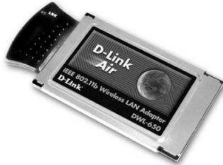
Figure 6.10: D-Link DWL-650 Prism2-based PCMCIA WLAN card used for testing attack
