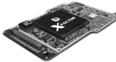
Figure 2.23: L3 Xfactor™ Selective Availability Anti-Spoofing Module (SAASM)
