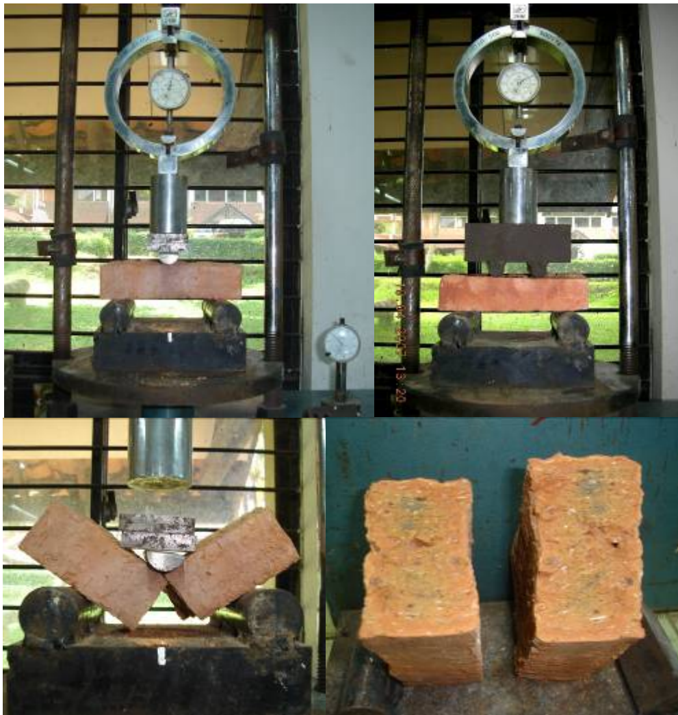
Figure 3.20 Tests set up for determining the modulus of rupture
