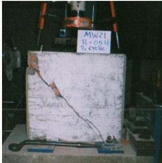
Figure 4.25 Failure type of wall MW21
