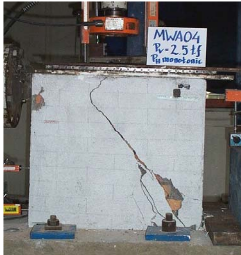
Figure 4.69 Failure pattern and load-displacement of wall MWA04
