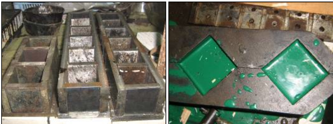
Figure 3.7 Moulding apparatus for 50 mm × 50 mm × 50 mm mortar cubes
