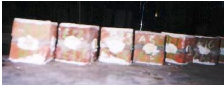
Figure 3.13 Compressive brick specimens after capping
