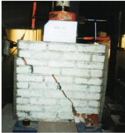
Figure 4.12 Failure pattern of wall BW09
