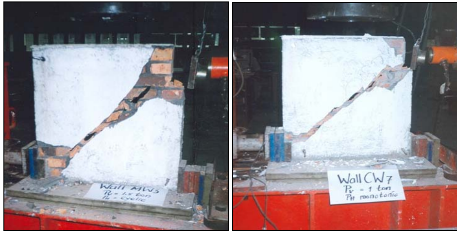
Figure 4.6 Wall failure pattern caused by lateral loads
