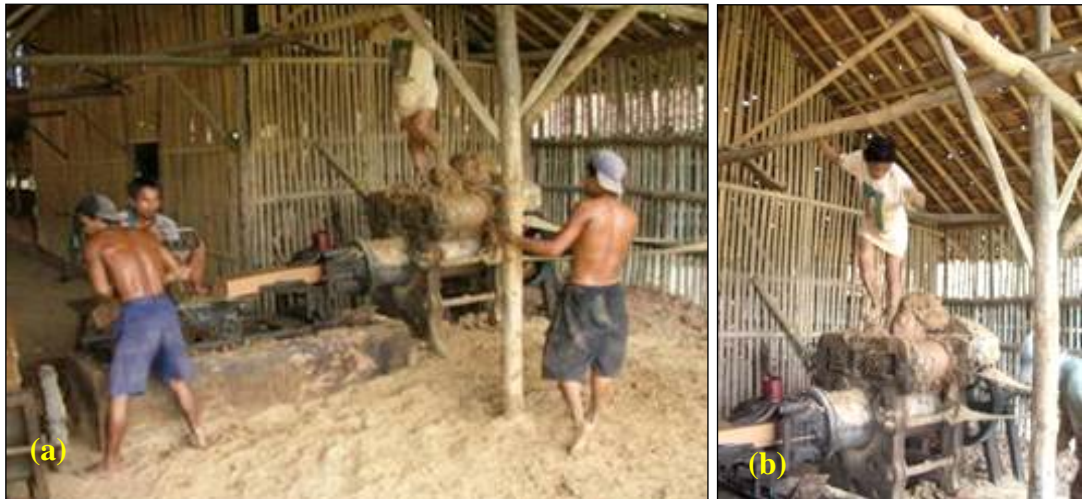
Figure 2.21 Moulding process (a) Labourers working with moulding machine, (b) Blending raw dough
