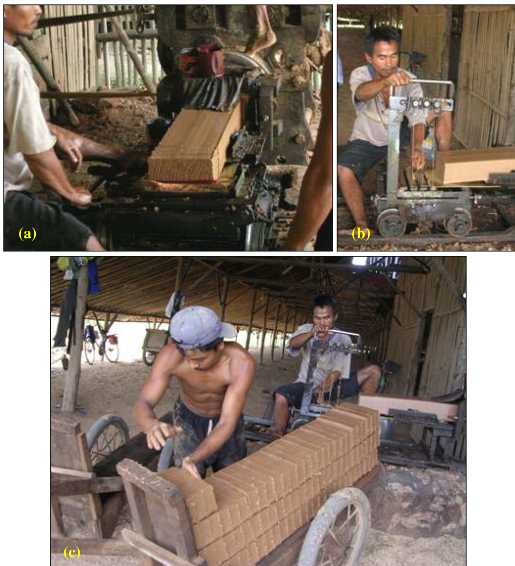
Figure 2.22 Wet brick cutting process (a) Brick forming, (b) Manual cutting, (c) Manual collection for transporting
