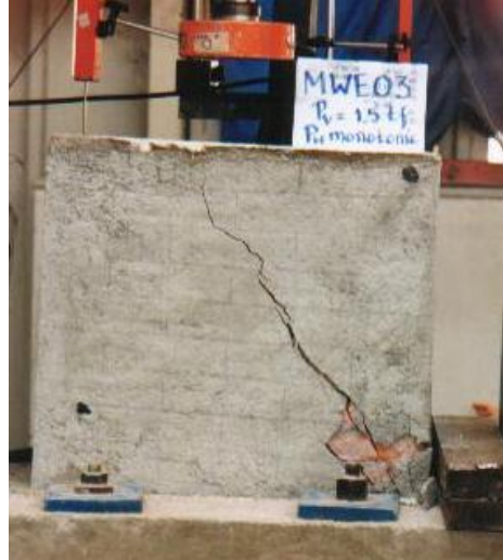
Figure 4.88 Failure pattern of wall MWE03
