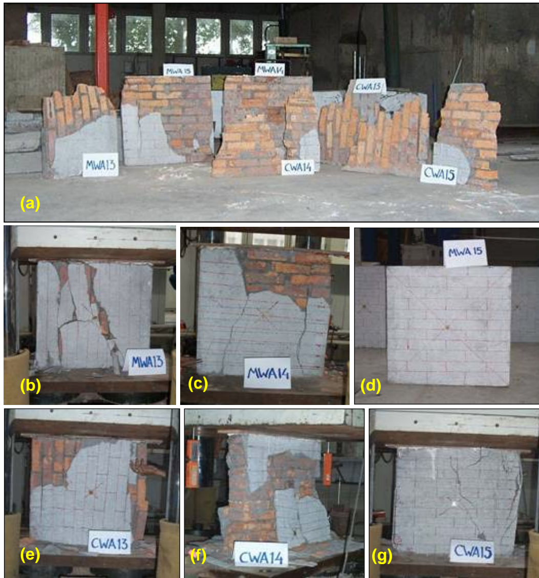
Figure 3.42 (a) to (c) Failure pattern of compressive wall MWA and CWA (d) Wall MWA before testing, (e) to (g) Mortar plaster failure of wall CWA
