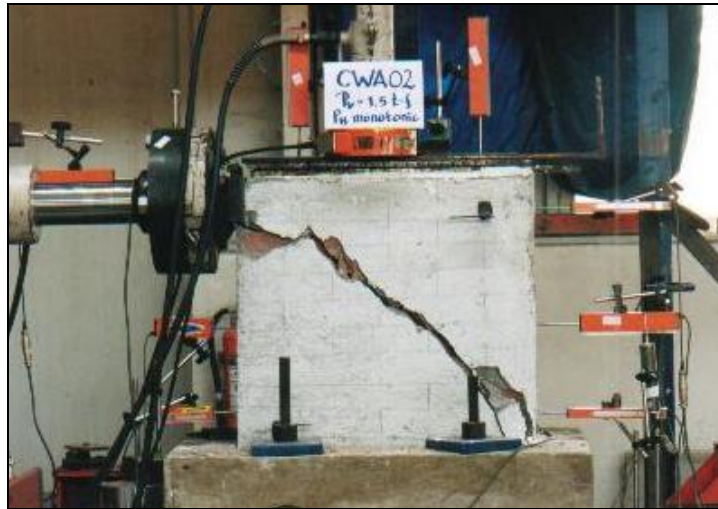
Figure 4.76 Failure pattern and load-displacement of wall CWA02
