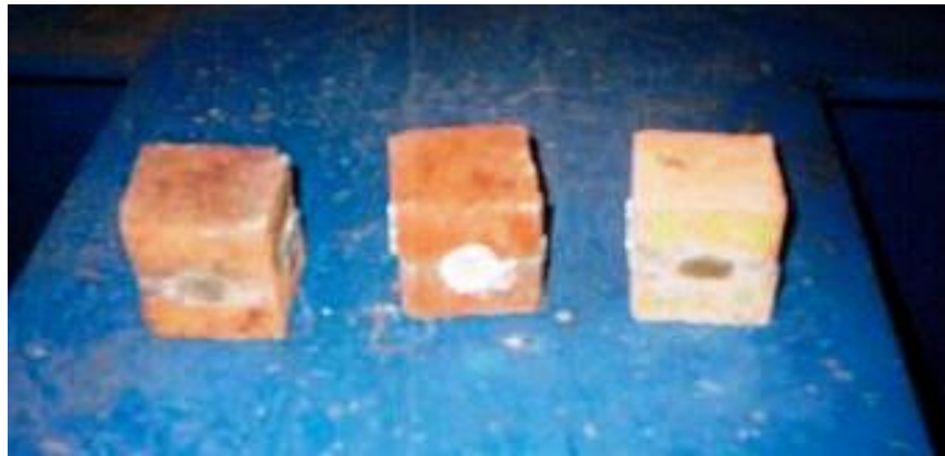
Figure 3.12 Compressive brick specimens before capping
