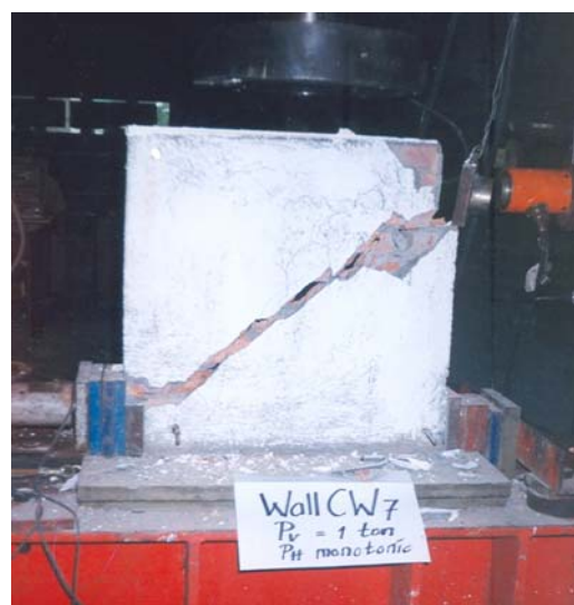
Figure 4.41 Failure type of Wall CW07
