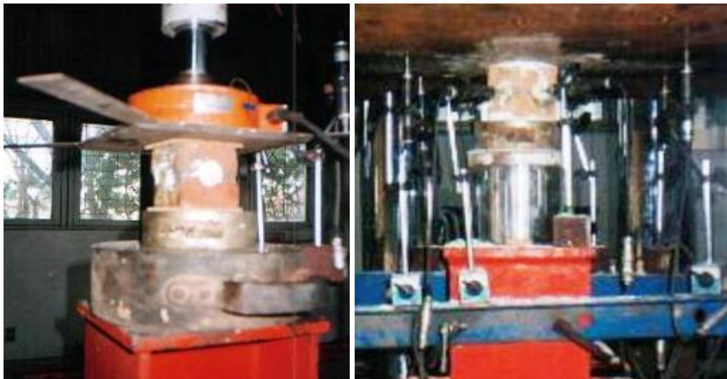
Figure 3.14 Compression test on brick specimen without and with LVDT configuration
