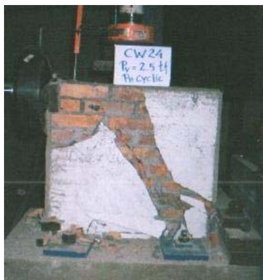
Figure 4.58 Failure pattern of wall CW24
