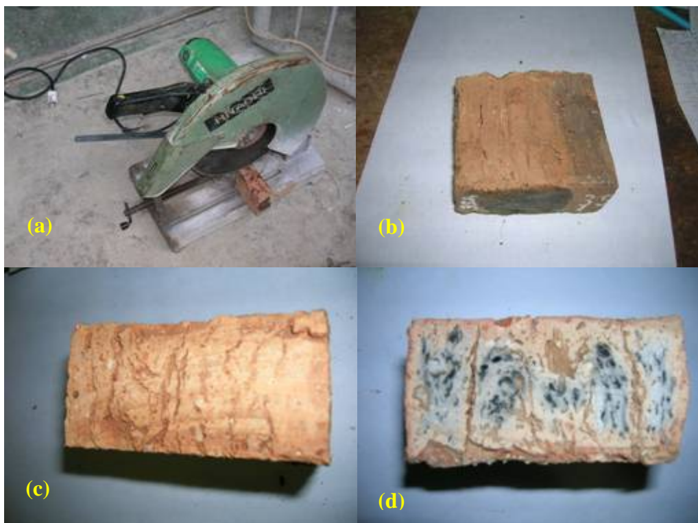
Figure 3.11 (a) Cutting Machine, (b) Half part of unit brick, (c) Cross section area of brick, (d) Cross section area of over burnt brick
