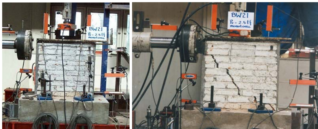
Figure 4.20 Wall BW 21 before and after testing
