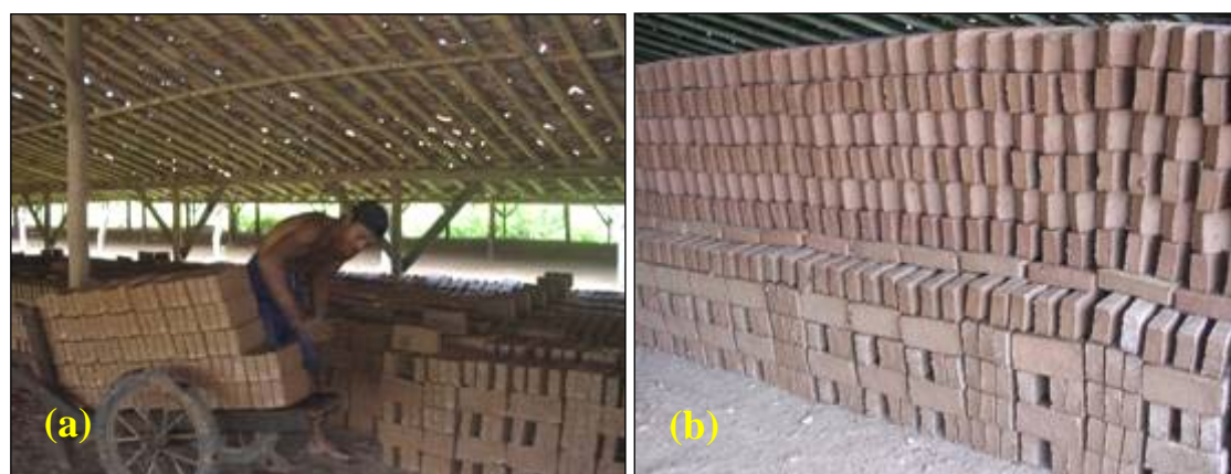
Figure 2.23 Treatment for natural air drying process (a) Transporting wet bricks, (b) Air drying process in lio
