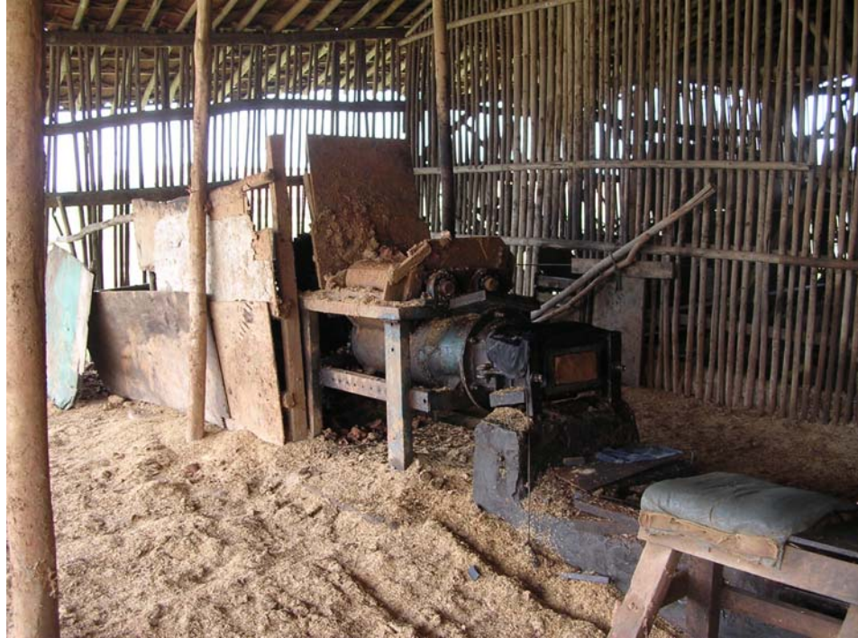
Figure 2.20 Machinery apparatus for pressing the brick paste
