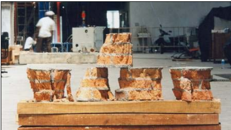
Figure 3.29 Failure type of short brick column specimens
