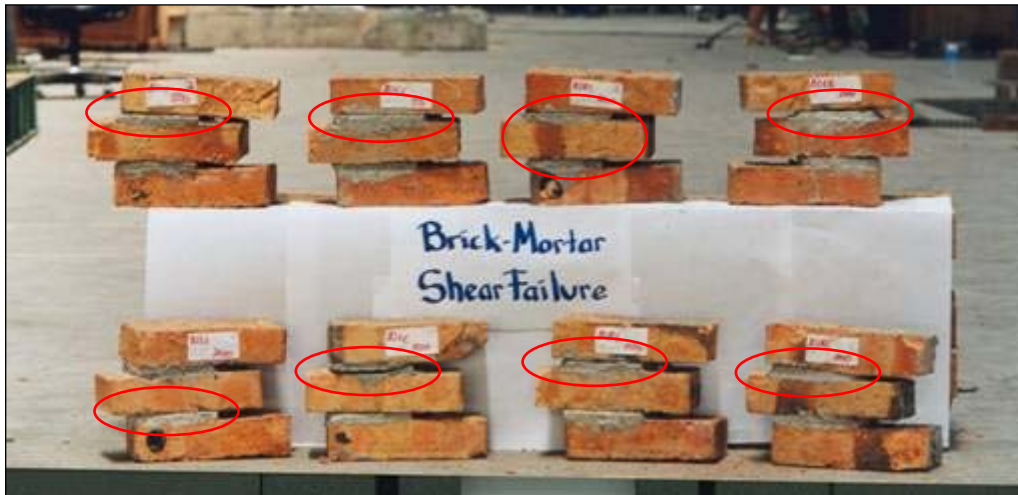
Figure 3.26 Triplet specimens after testing with slip failure pattern
