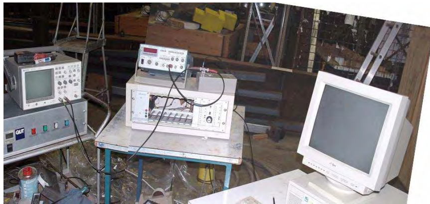
Figure 3-18: Frequency generator, oscilloscope, actuator controller, pump controller and data acquisition computer
