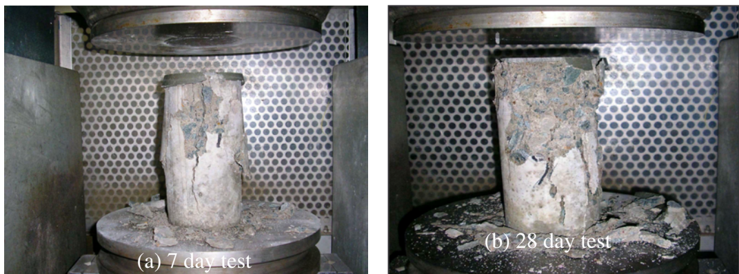
Figure 3-25: Typical failure pattern of the concrete compressive strength
