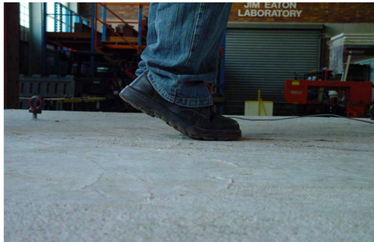
Figure 3-21: Heel impact excitation
