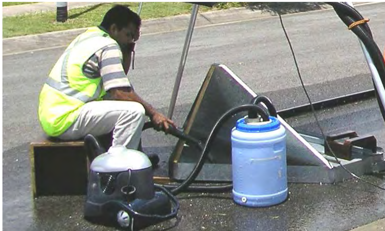
Figure 4.10 – Collection of runoff samples to polyethylene containers
