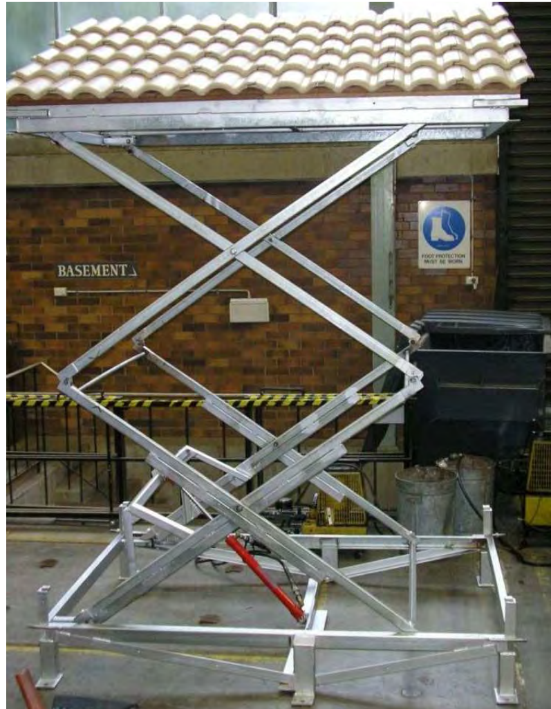
Figure 3.10 – Concrete tiled model roof mounted on scissor lifting arrangement
