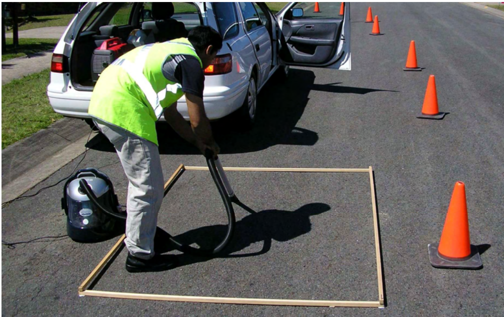
Figure 4.7 - Dry sample collections from road surface plots
