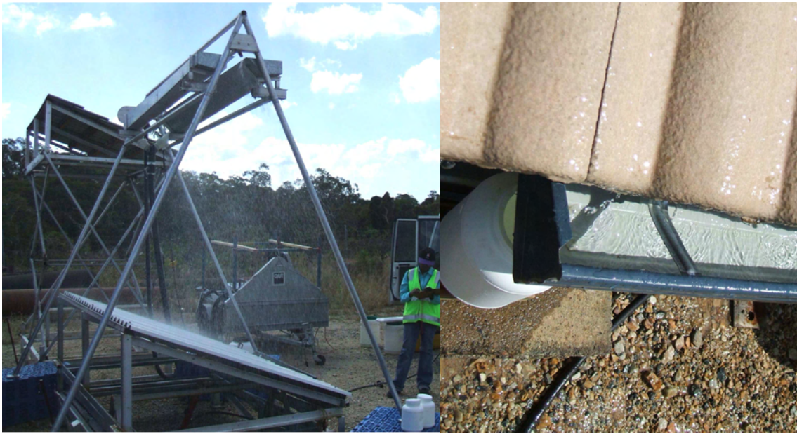
Figure 4.11 – Rainfall simulation on roof surfaces
