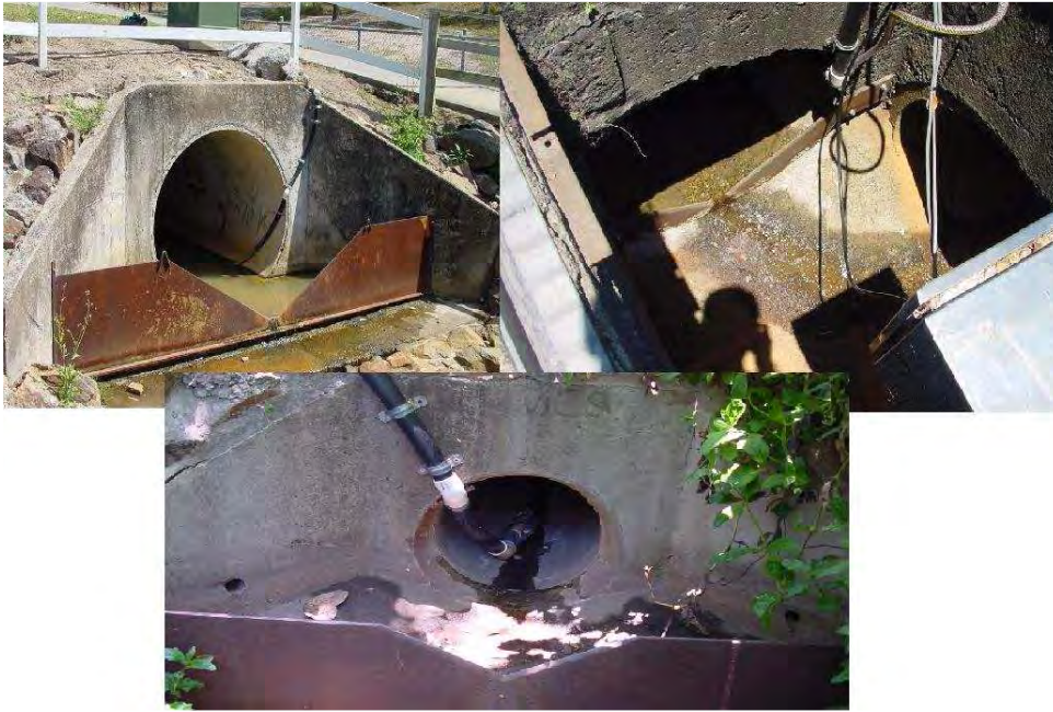
Figure 4.4 - Depth gauges and V-notches at the three catchment outlets
