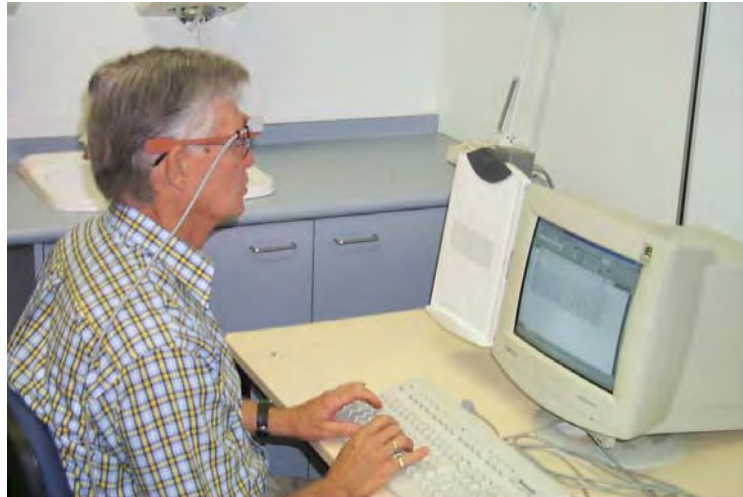
Figure 6.1 Set-up of Polhemus Inside-Track system for the copy task. The transmitter cube is the grey box at the top rear of the copy holder to the left of the monitor; sensor cube is mounted on the spectacle frame and is visible just in front of the right temple.
