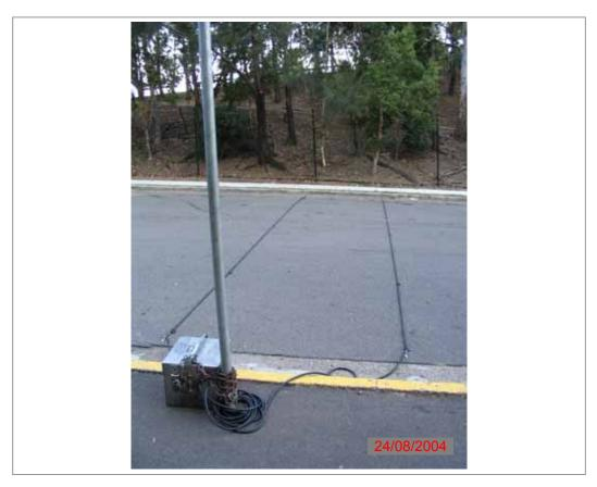
Figure 6.10 – Typical installation of the automatic traffic counter
