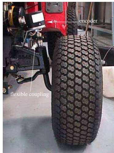
(a) The absolute encoder measures the rotation of the front left-hand wheel.
