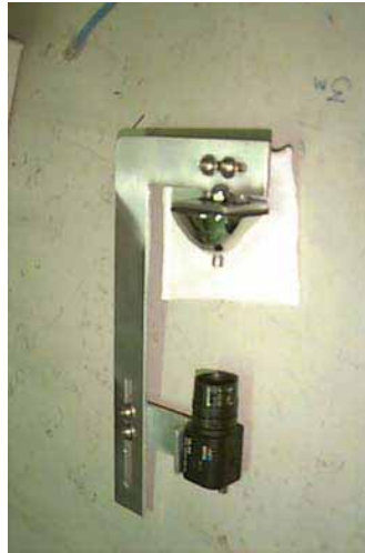
(a) A catadioptric omnidirectional system.
