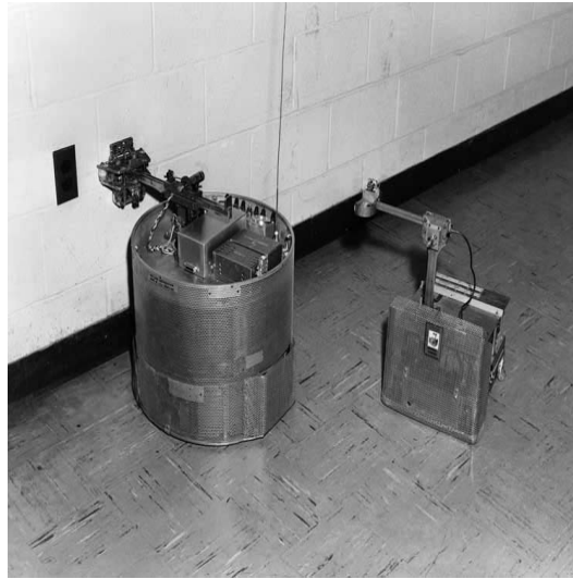
Figure 2.2: Two versions of the Hopkins ‘beast’, the larger of which is re-charging at the wall socket. Image courtesy of the Robotics Institute at Carnegie Mellon University http://frc.ri.cmu.edu/~hpm/book97/index.html .
