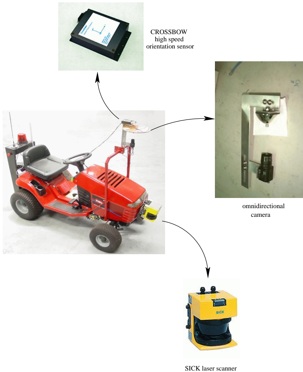
Figure 4.14: An overview of the AT's sensors.
