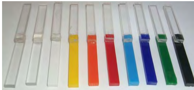
Figure 9.15: Specimens cured with light sensitive adhesive for two seconds
