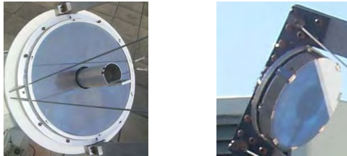
Figure 4.2: Primary and secondary mirrors
