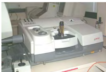
Figure 4.10: FTIR spectrometer Thermo Nicolet Nexus
