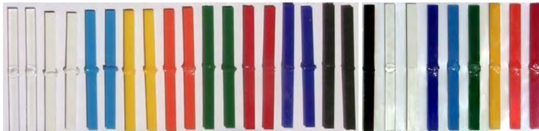
Figure 8.9: Identically colored specimens butt joined with imaging optics
