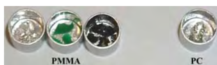
Figure 5.27: PMMA and PC samples used for DSC
