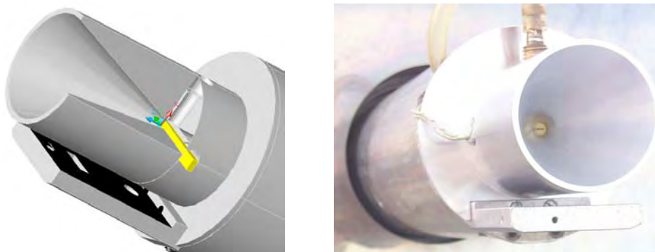
Figure 9.5: Specimen mounting – a sectional view and a photograph
