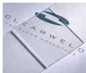
Figure 3.11: Clear PMMA lap joint made with ClearWeld absorber at the interface
