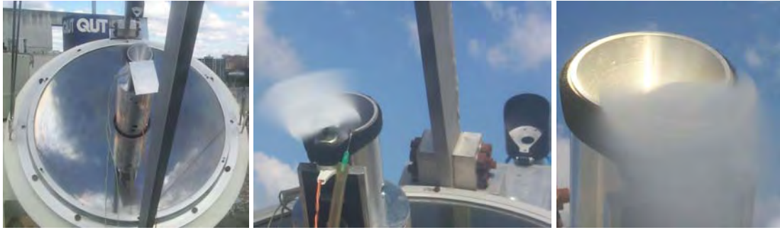
Figure 7.24: Provisional light chopper and experimental mist/smoke maker
