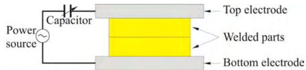
Figure 3.5: Radio-frequency welding set-up
