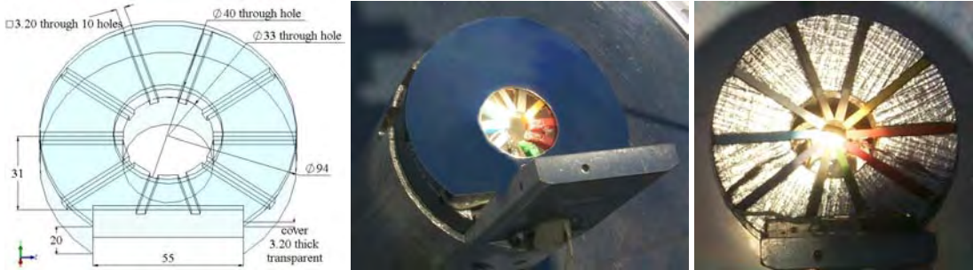
Figure 5.31: Design drawing and pictures of holder with all irradiated specimens
