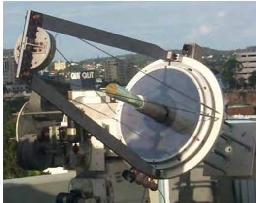
Figure 7.13: Overall view of the SEC with the truncated cone concentrator
