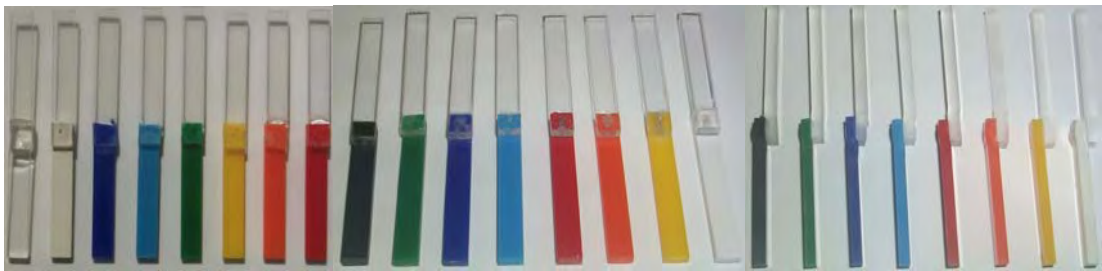
Figure 8.25: Lap joined specimens using non-imaging optics
