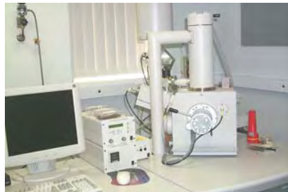
Figure 4.13: JXA-840A scanning electron microscope
