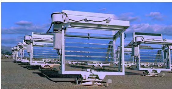
Figure 3.24: EMMAQUA and ACUVEX Fresnel concentrator weathering devices
