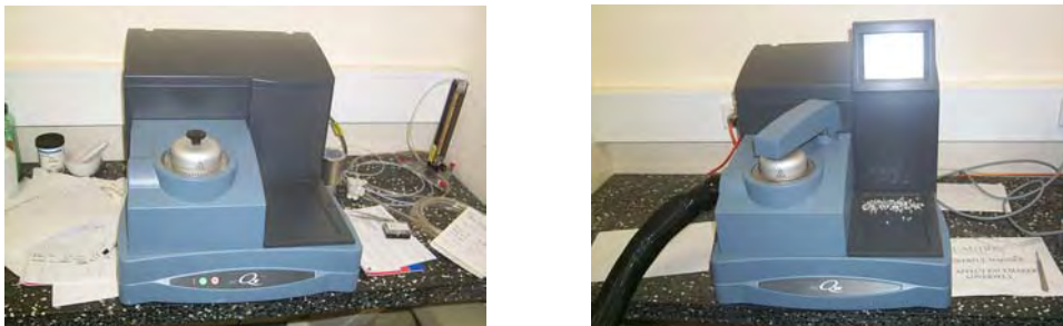
Figure 4.11: Differential scanning calorimeters TA Q10 (left) and TA Q100 (right)
