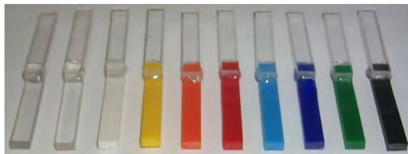
Figure 9.14: Specimens cured with light sensitive adhesive for 60 seconds
