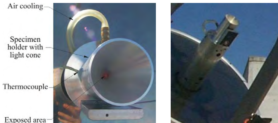
Figure 7.23: Cooling inlet in the provisional third stage concentrator
