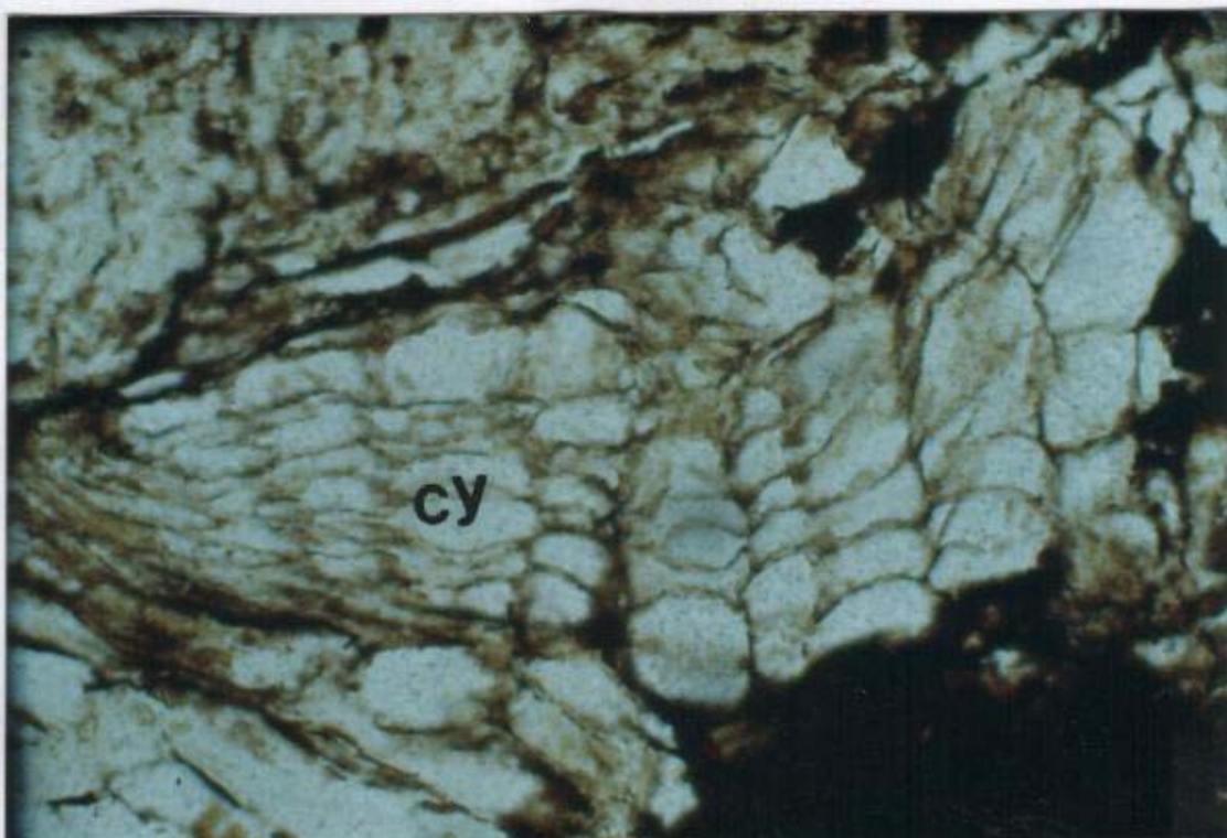
Photograph 36: Clay pellets (CY) in coal (thin section, transmitted light) (Sample No. TH19, Westfalen No. 3 mine, Blackstone Formation-coal as sold, February 1973).
