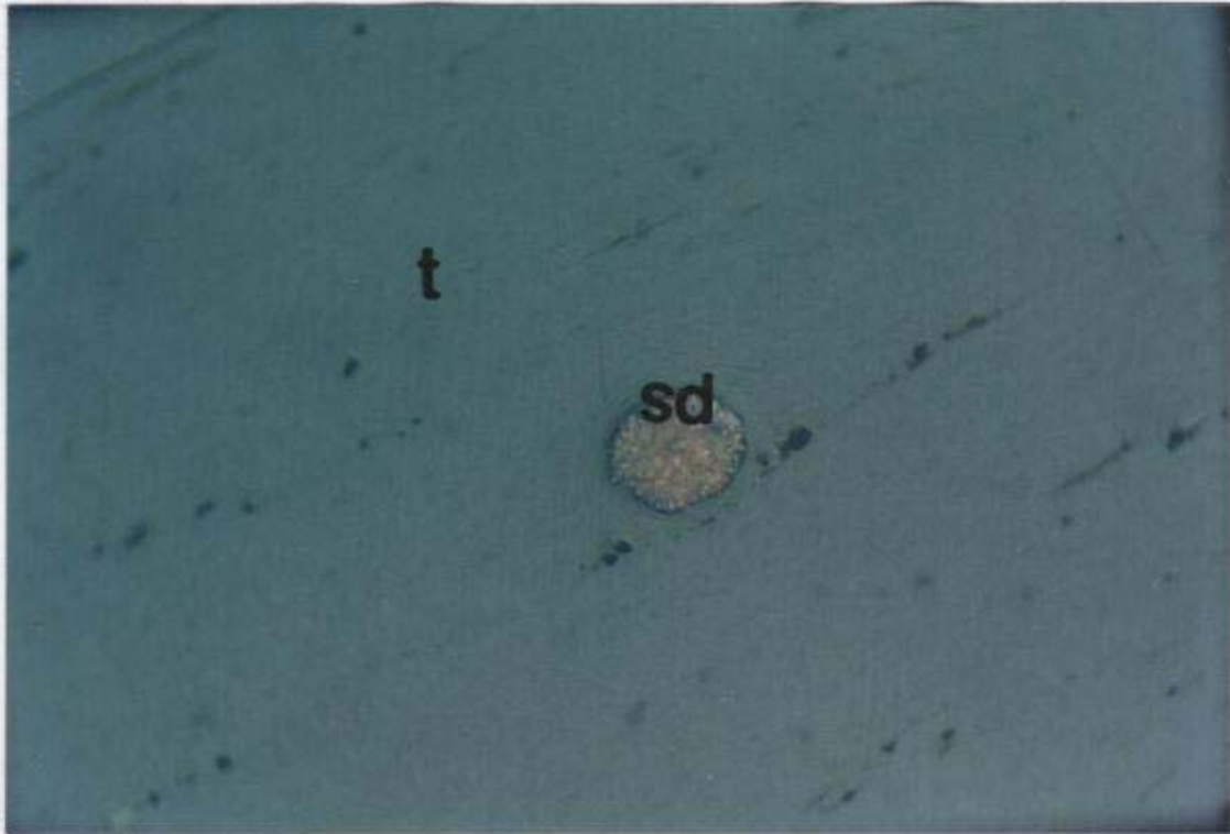
Photograph 1: Sideritic micro nodule (centre) in telovitrinite (Sample No. G1, North Ipswich-Haighmor and Moreton Extended mines, coal as sold).
