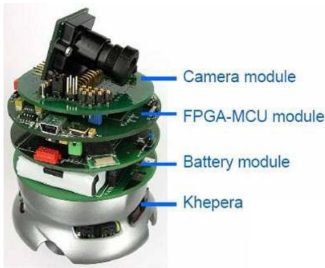
Fig. 9. Vision system attached to the top of the minirobot Khepera (courtesy of SCT-University of Paderborn)
