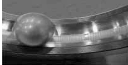
Fig.5. damages on the bearing (source: ABB technical guide)
