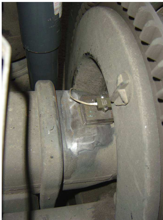
Figure 13. Accelerometer mounted on top of school bus axle.
