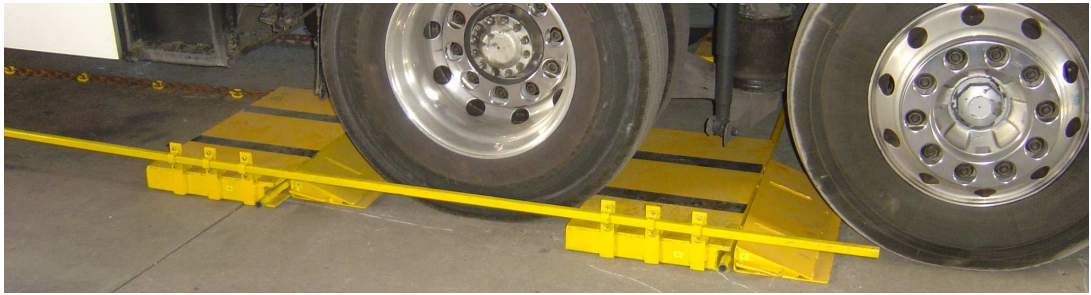
Figure 19. Before: showing preparation for the step test on the coach.
