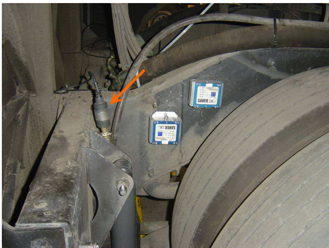
Figure 15. Air pressure transducer (arrowed).
