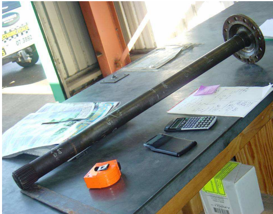
Figure 24. Calculating the half-shaft mass outboard of the strain gauges.
