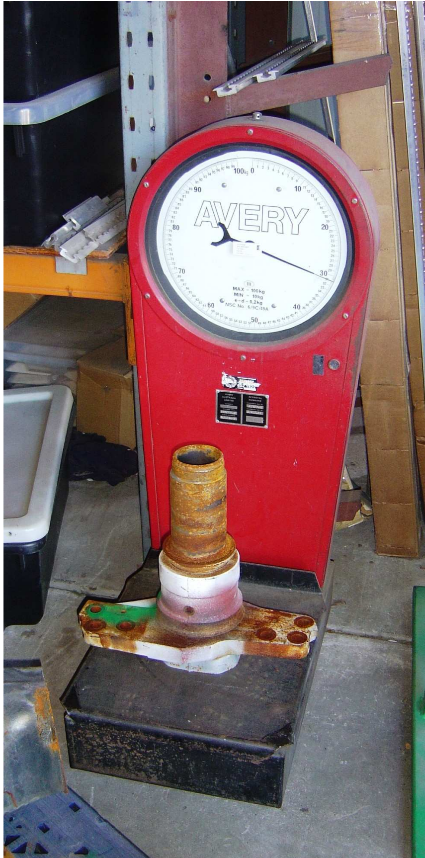
Figure 26. Weighing the drive axle housing mass outboard of the strain gauges. This photo shows the coach axle portion.
