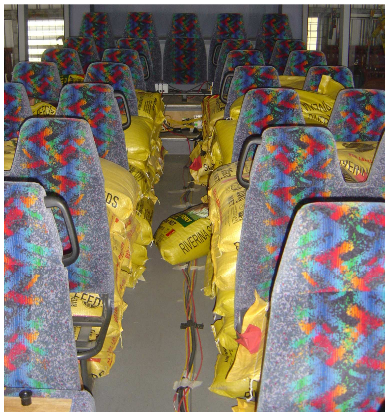
Figure 7. Sacks of horse feed (yellow) used to achieve test loading on the buses.
