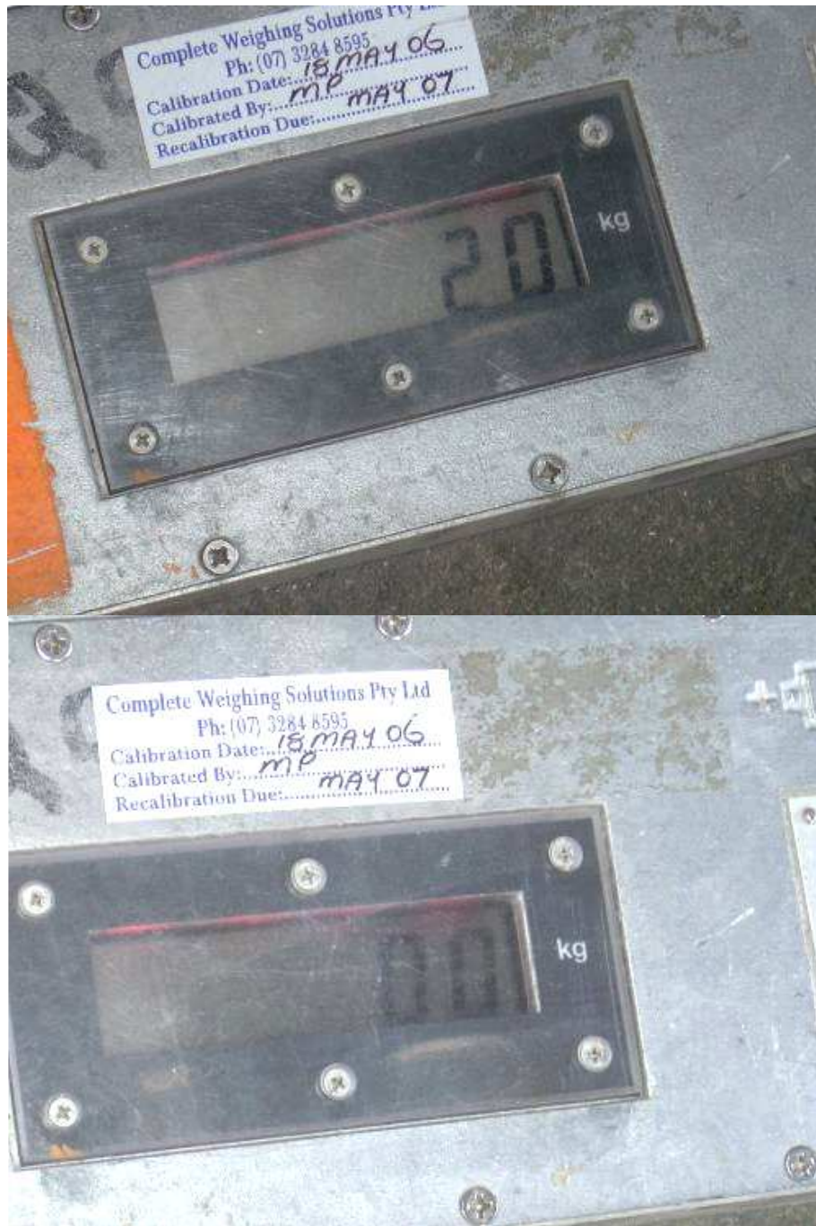
Figure 30. Gradually reducing the wheel force as the chassis is jacked up: top panel, almost there; bottom panel, no wheel force.
