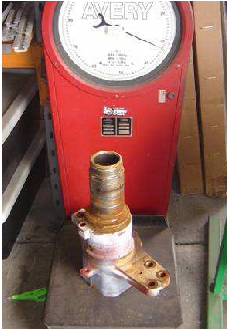
Figure 25. Weighing the drive axle housing mass outboard of the strain gauges. This photo shows the bus axle portion.
