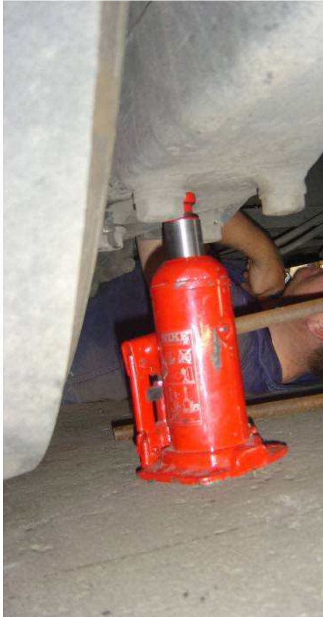
Figure 29. Jacking the test vehicle so that the static wheel-force could be set to zero.
