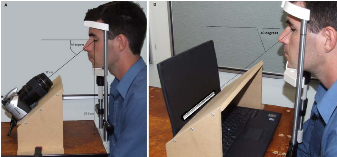
Figure 1: A) Camera and subject fixating at 40° downward gaze; B) Visual task positioned at 40° downward gaze, approximately 40 cm from the subject.
