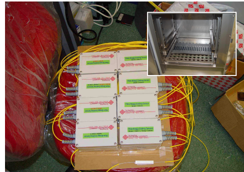
Figure 1 Packaged FBG strain gauges boxed in ABS enclosures with two 3 mm fiber outlets (Inset shows the FBG sensors epoxied on nitinol sheets in an oven after baking at 80°C for 5 hr)
