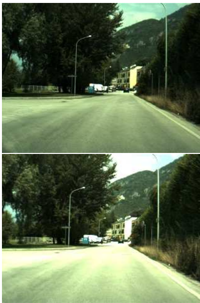
Figure 1: Difference caused by camera bias.
