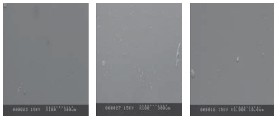
Figure 2. Scanning electron micrograph of a spun-cast pHEMA lens. Front surface (left) (original magnification x100), back surface (centre) (original magnification x100) and high magnification front surface (right) (original magnification x3000).
