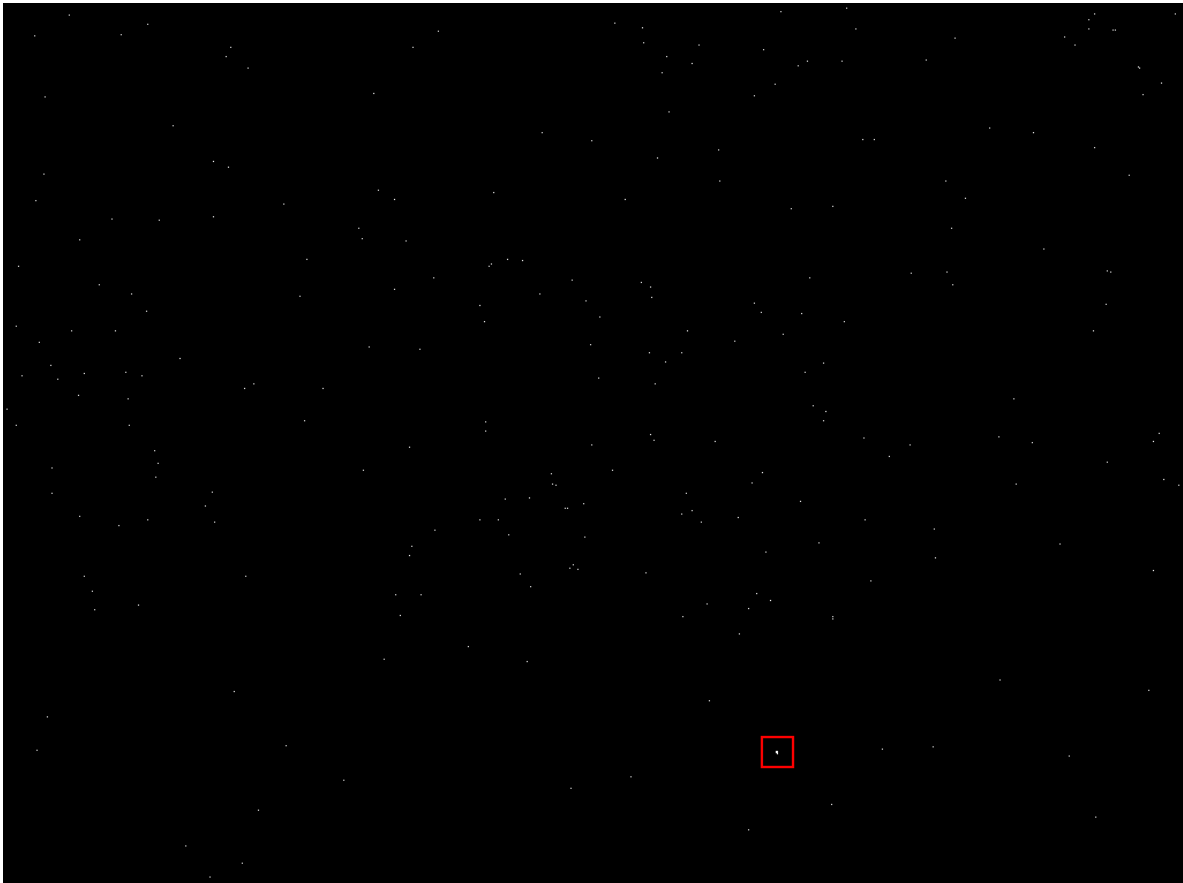
Fig. 6(d): Binary representation of CMO filter output showing detected target & false alarms
