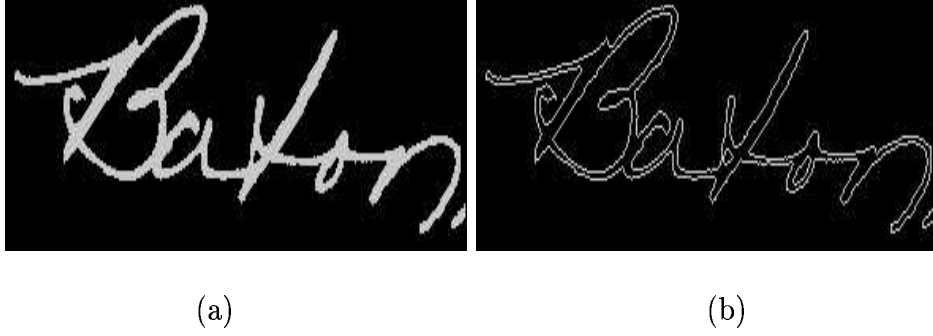
Figure 3: Examples of edge detection. (a) binarized image; (b) edge of the binarized image.
