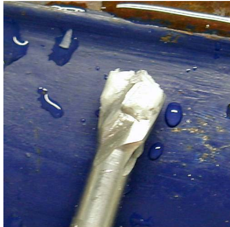
Figure 3 Swarf repeatedly re-accumulates in front of leading edge of drill tip when performing end cutting procedures. Note the flutes running down the body of the bit are clear of debris due to favourable helix angle.
