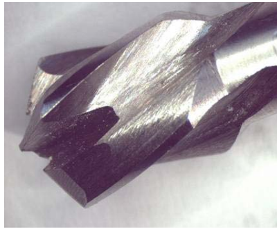
Figure 2 Reamer Tip. Note the difference between negative rake angle established at the centre cutting area of the drill compared to positive helix angle of the drill body.
