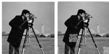
Fig. 3. (Left) Copy-attacked Cameraman stego image. (Right) Tampered regions highlighted by fragile watermark detection
