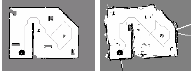
Fig. 6. Completed Maps (a) Simulation (b) Real Robot
