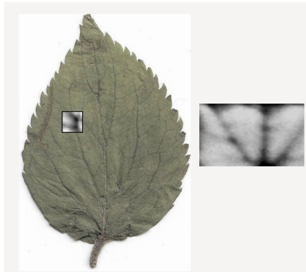
Figure 2.4: The image on the left shows a photograph of a leaf with a small THz image superimposed on top. The image on the right is a large area THz image of a different leaf, where the vein structure can be clearly seen.
