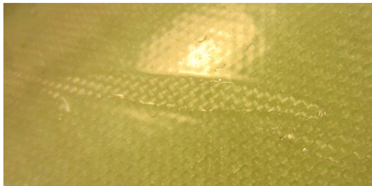
Figure 6.19. Detail of a bubble defect on the epoxy.
