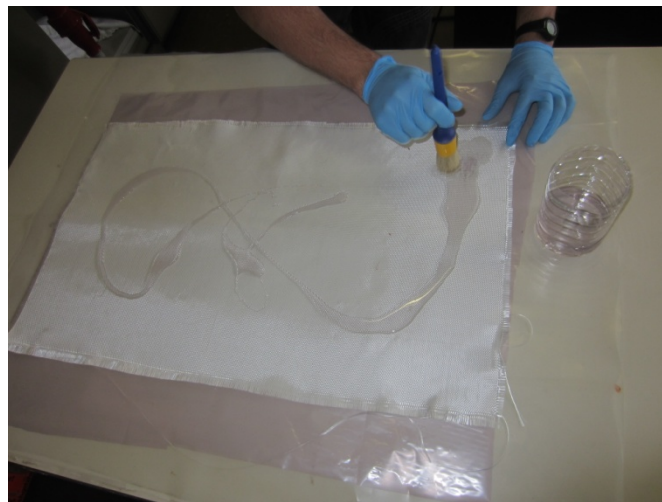
Figure 6.17. Impregnation of the fiberglass with epoxy.
