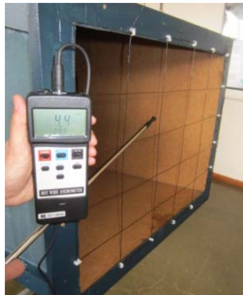
Figure 4.6. Grid at the wind tunnel exit.
