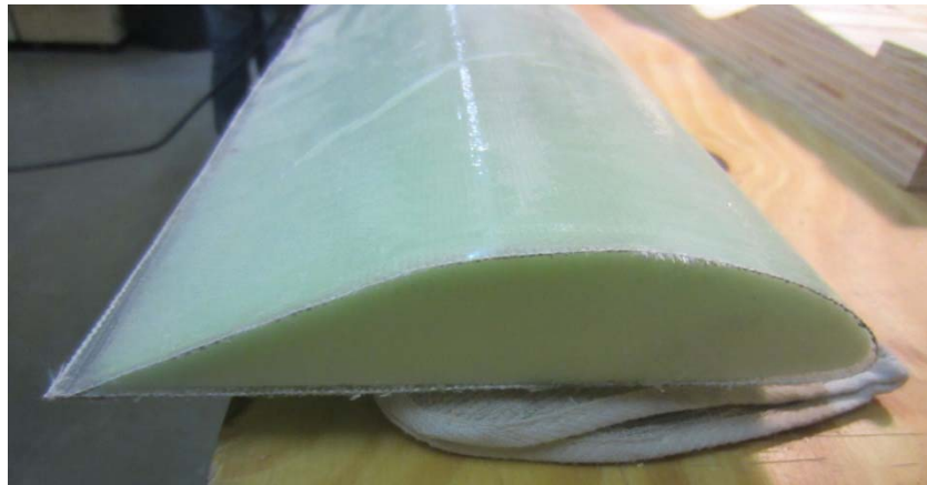
Figure 6.10. Foam core with the fiberglass and epoxy layer.
