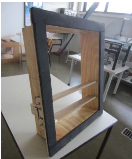
Figure 4.19. Airflow redirecting device.
