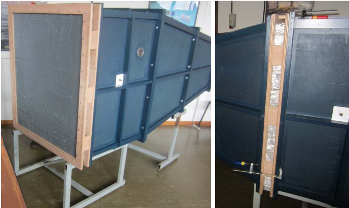
Figure 4.12. Honeycomb installed in the wind tunnel.
