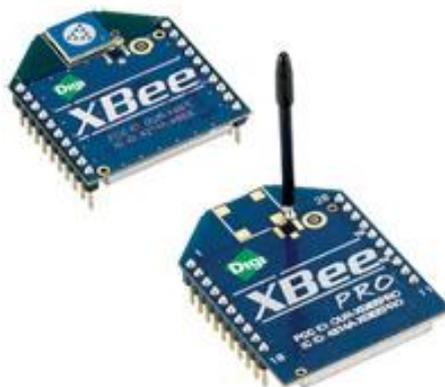
Figura 2.13: Chip XBee
