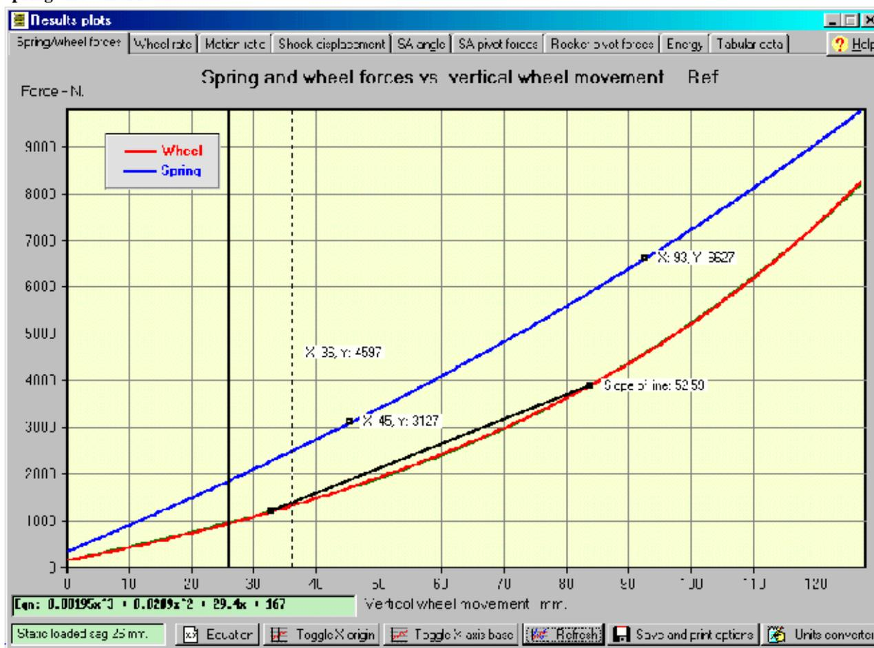
These curves show the actual forces experienced by the wheel and shock spring, over the range of wheel movement. In actual use there will be additional forces due to damping, but these vary with shock velocity and so cannot be calculated in a static analysis such as this. These curves and that of the actual wheel rate are probably the most important in any suspension analysis. If specified, the effects of a bump-stop rubber will be shown in these plots.
