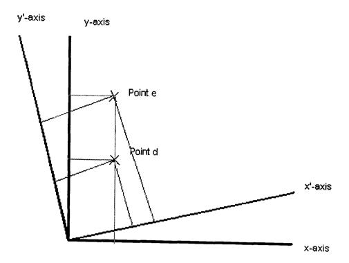
What the diagram shows is that for any two points, d and e, although it is possible to rotate the (x,y) axis to (x',y'), and hence effect a co-ordinate transformation from (x,y) to (x',y'), it is not possible to alter the separation between points d and e simply be rotation of the axes. Plainly the distance between the two points is invariant, although the distances between the two points as defined in terms of the x and y coordinates obviously vary according to the frame of reference.
