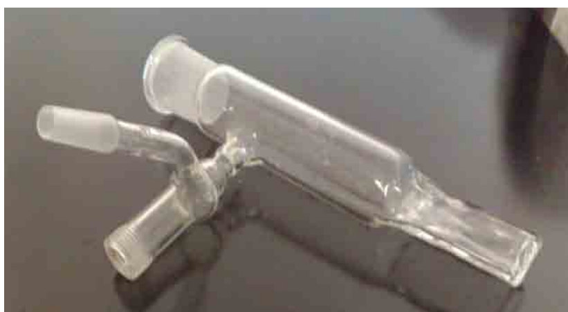
Figure 5-19 Flat compartment flask for modification of silicon wafers with 1,8-nonadiyne
