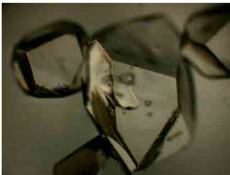
Figure 6-8 Typical habits of BHT crystals (magnification 100 \times ), crystallization from ethanol
