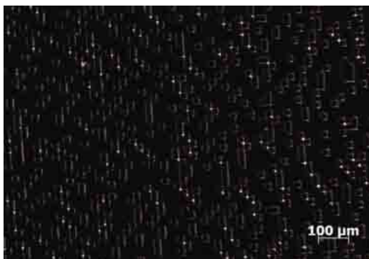
Figure 6-20 Optical microscope image (episcopic illumination) of the master used for microcontact printing of the thiols
