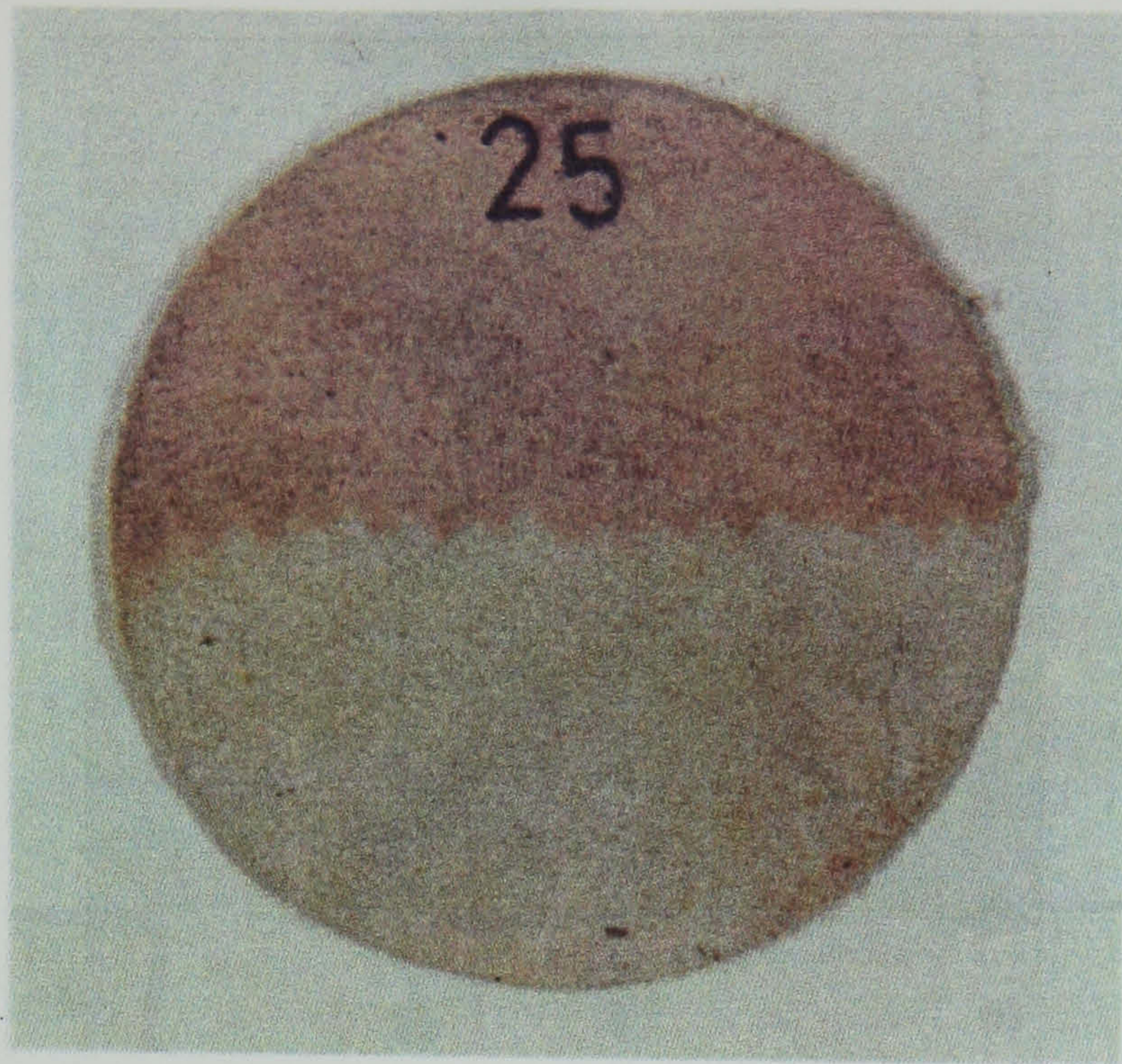
Figure 2.13 A test sample after being skived using the static matrix method.
