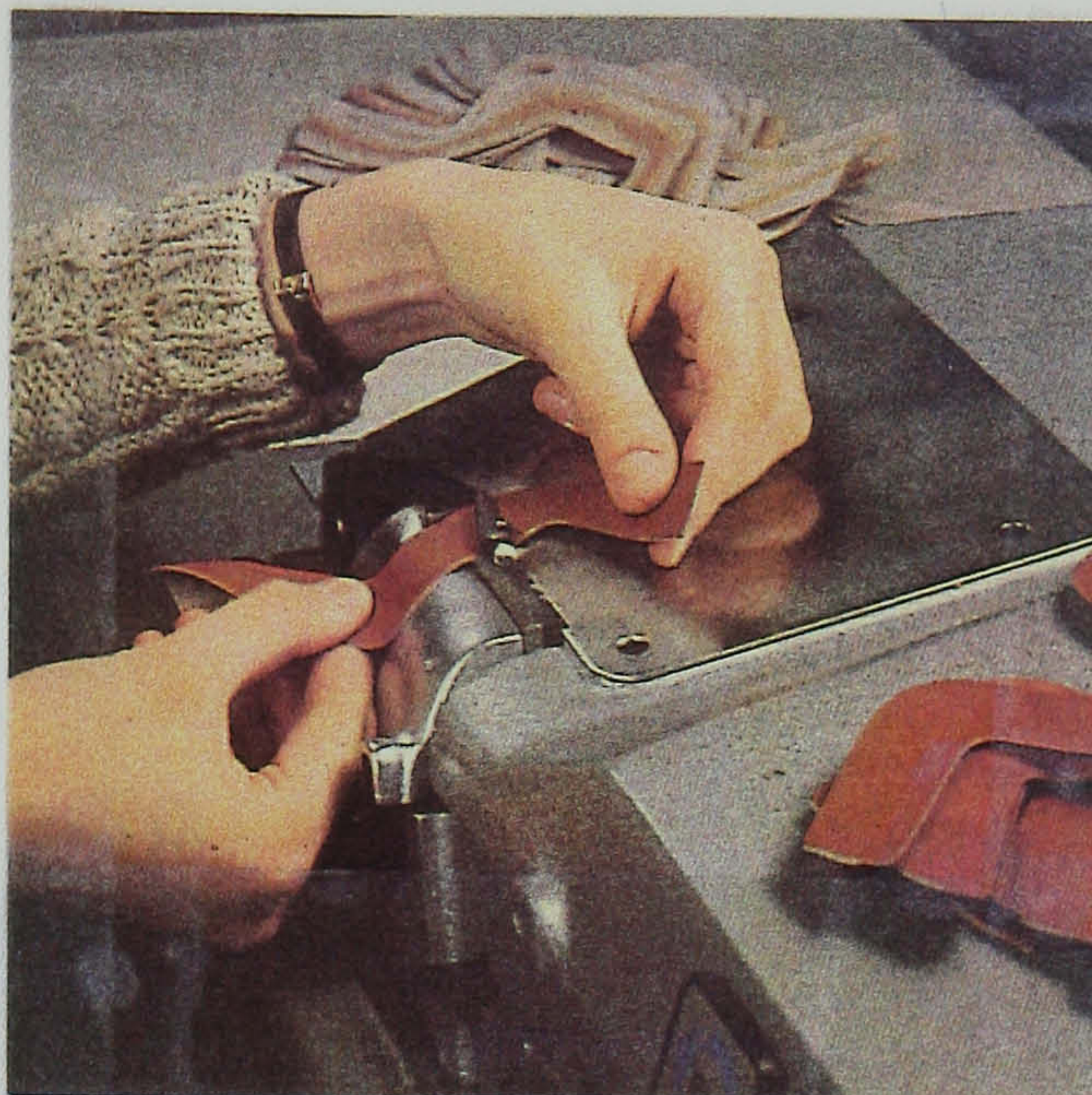
Figure 1.4 A close-up view of skiving operation (By permission, BUSM Ltd.).
