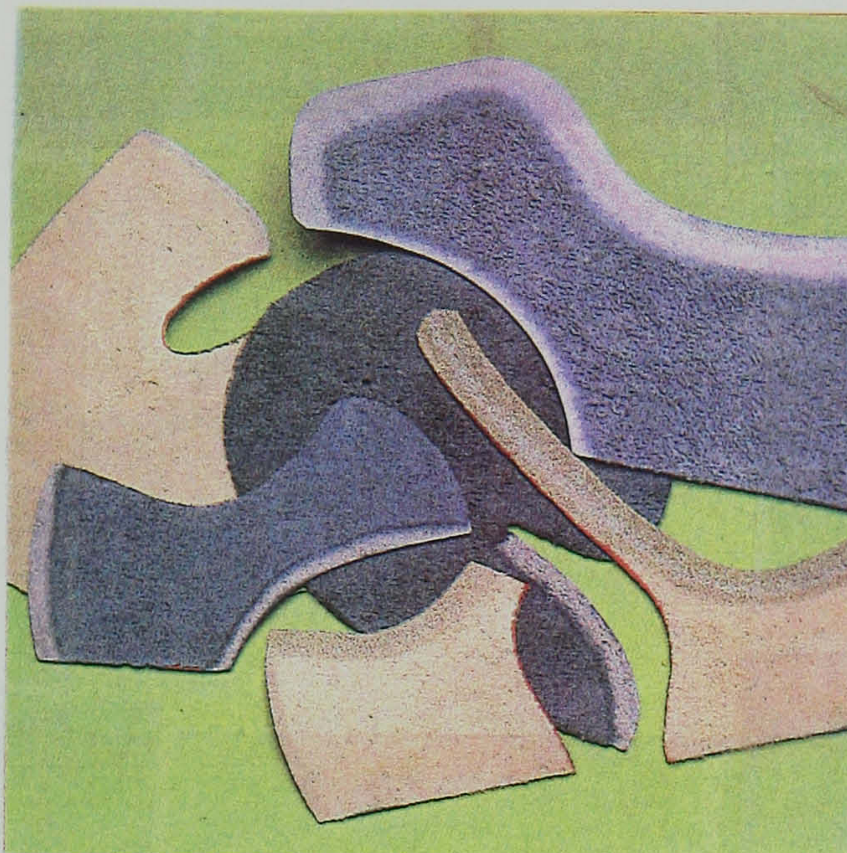
Figure 1.6 Examples of skived components (By permission, BUSM Ltd.).
