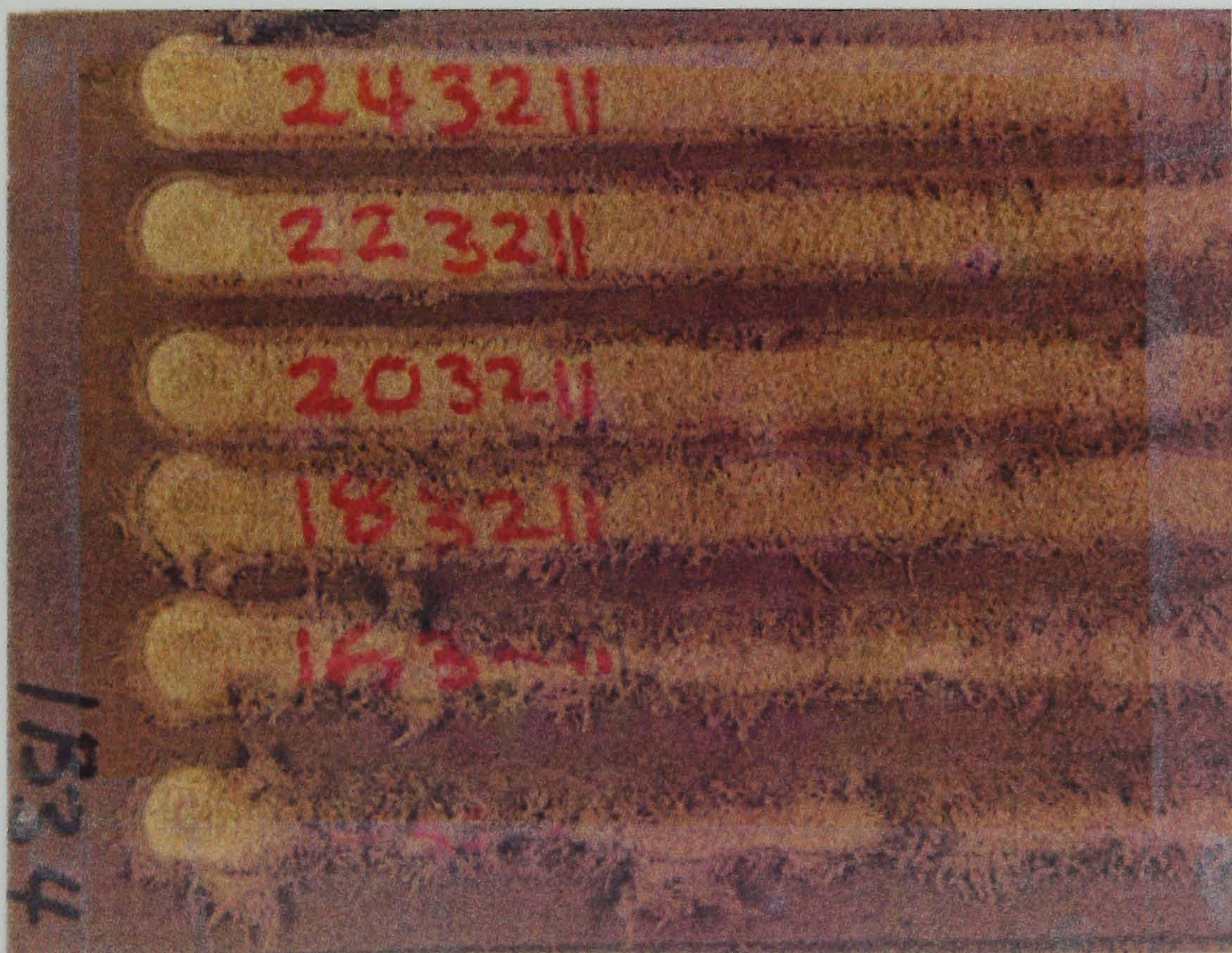
Figure 5.16 Photograph of a typical test sample with poor machined surface quality.
