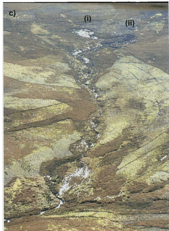
Figure 5.15. Slope channel-coupling at North Pennine peat slides. a) Middlehope, almost all displaced material discharged directly into gully head. (Note shallow slope failures visible on gully sidewalls, may indicate localised tendency for slope instability); b) Langdon Head, upper rafts stabilised (i), but lower scar (ii) largely excavated into Langdon Beck beneath. The scar probably occupied a former gully head; c) Feldon Burn, twin scars (i and ii) feed extensive channelised track.
