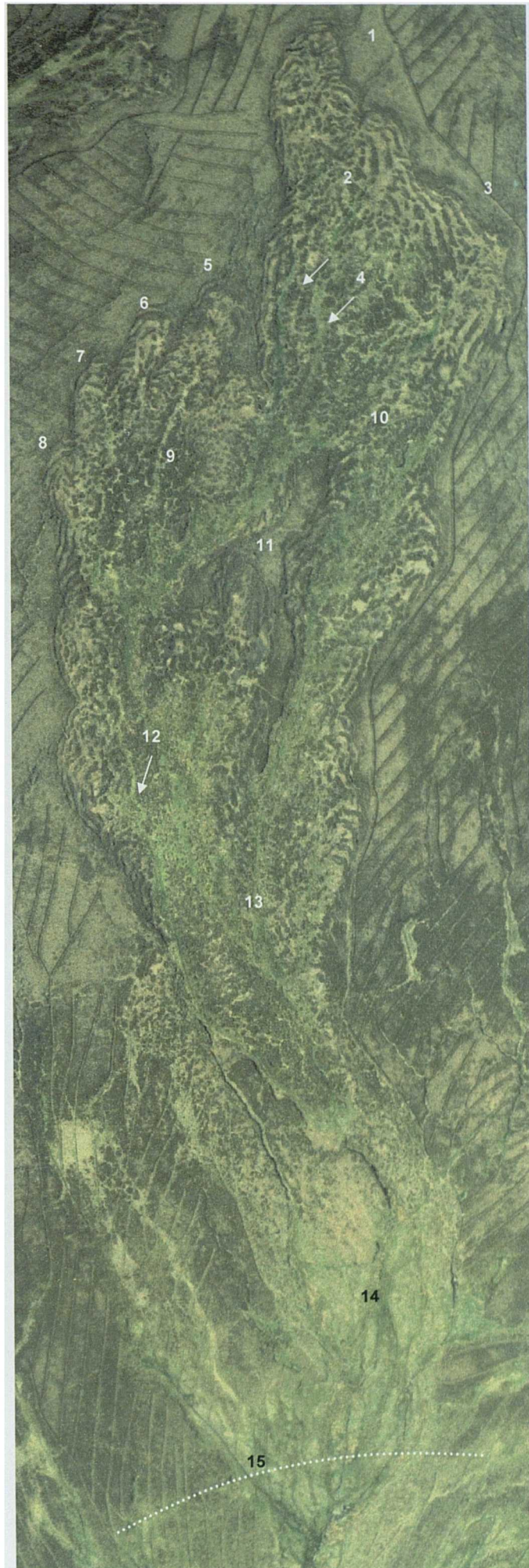
Figure 8.1. An aerial photograph of the Glendun bog burst, illustrating key morphological features (Photo taken in 1999, failure occurred in 1963).
