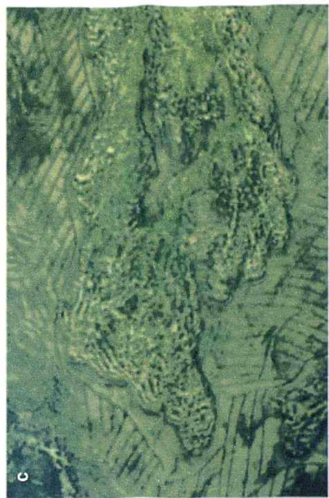
Figure 2.8. Depositional and scar morphology at bog burst sites: a) The Geevagh (Straduff) bog burst (1984), disturbed crescentic rafts separated by deep tears are visible in the foreground, and narrowing of scar in the distance; b) similar arcuate tearing at Glendun (1963); c) an aerial photograph of the Glendun failure, illustrating distinctive rafting (dark) and tearing (light, cotton grass) patterns, and parallel grips.
