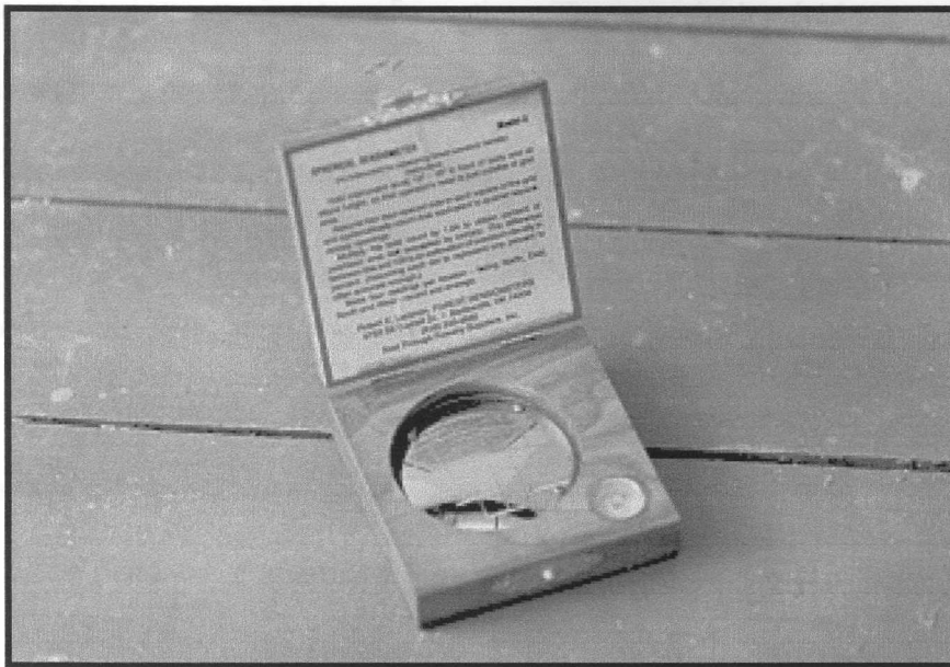
Figure 3.1: Densiometer used to measure canopy openness.
