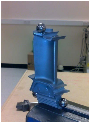
Figure 4.10 Fix a gas turbine using vice
