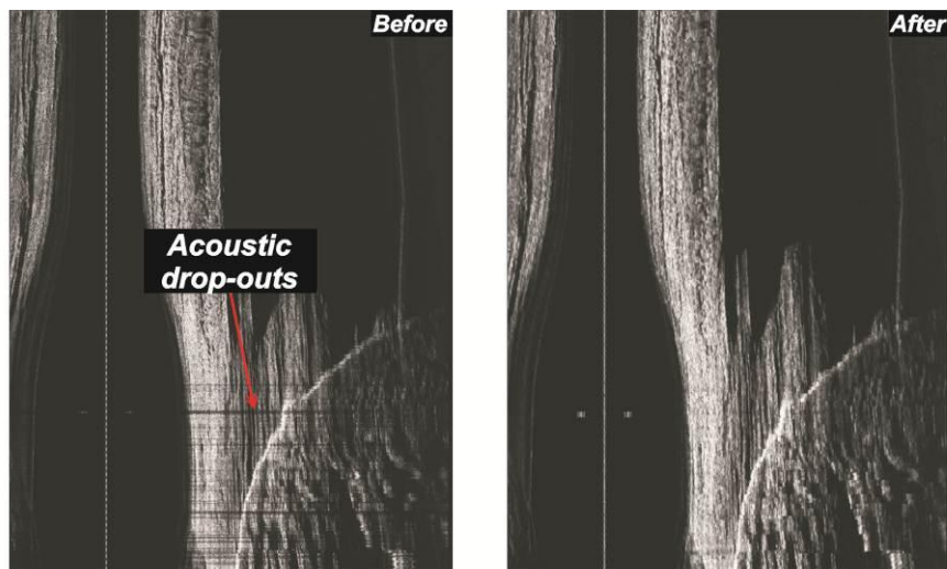
Figure 2.4.7 Acoustic drop-out suppression using PRISM. Drop-outs occur when vehicle yaw exceeds beam sensitivity (left image). Correction is mainly for aesthetic purposes. The final mosaic (right image) displays only very faint blurring where drop-outs have been removed by interpolation of adjacent sonar pings.
