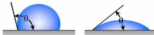
Figure 2.11 – Schematic representing the contact angle: it defines an hydrophobic surface when superior to 90^\circ (left), and an hydrophilic surface when inferior to 90^\circ (right) [24].
