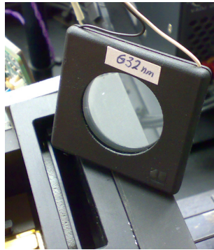
Figure 3.3 – FLC polarization rotator (Displaytech LV2525) removed from its holder.
