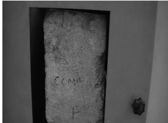
PLATE 4 Crushing test of one the sandcrete blocks.
