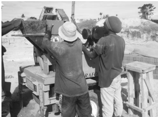
Pic 1: Making Hydraform blocks on the building site with a special machine. Source: Malaika Kids UK website.
