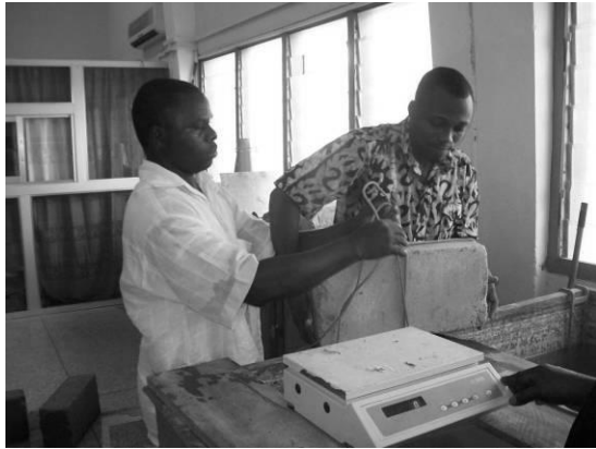
PLATE 3 Submerge the block in water to measure weight in water.
