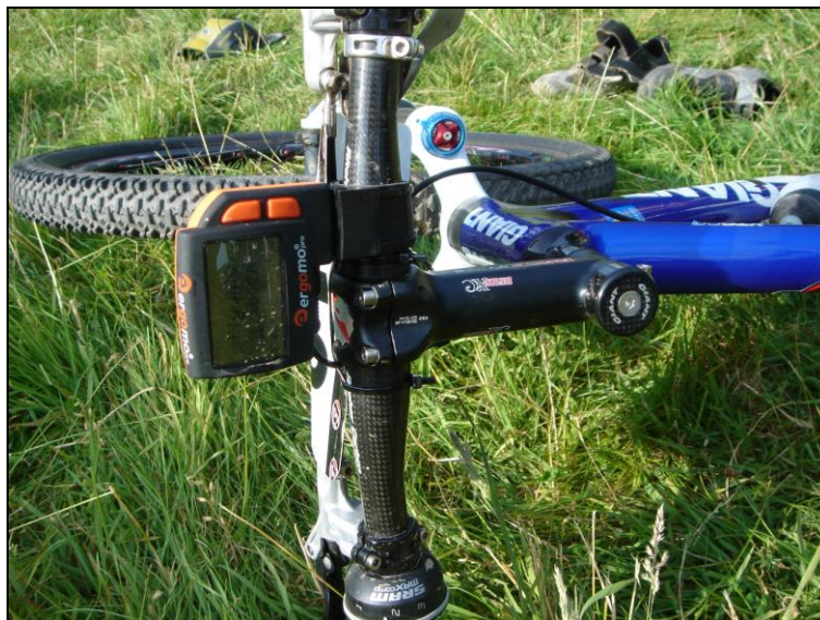
Figure Q.2: Participants' mountain bikes during a recovery period (left) and the Ergomo®Pro in situ (right).
