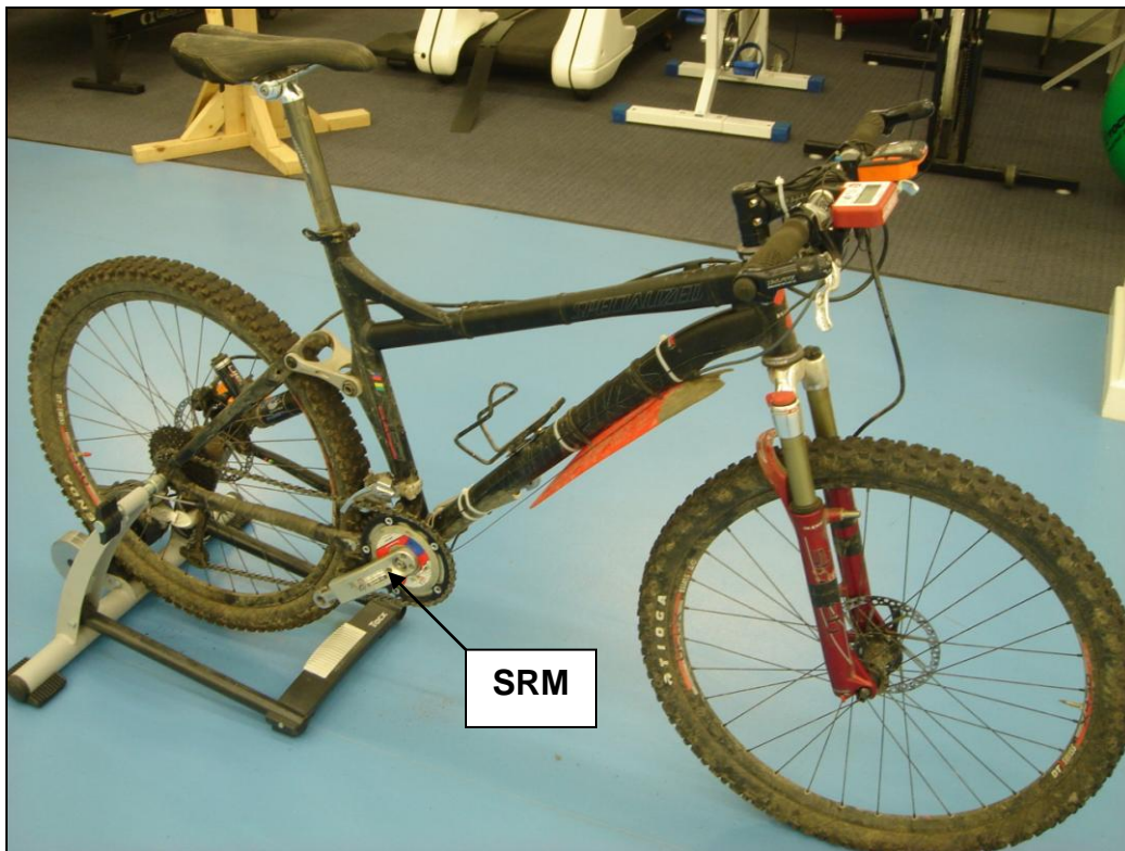
Figure 7.2: The mountain bike fitted with SRM and Ergomo®Pro power meters
