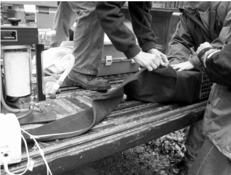
Figure 5. (b) The denim cone shown wrapped around the cage front and tightened with heavy duty Velcro.
