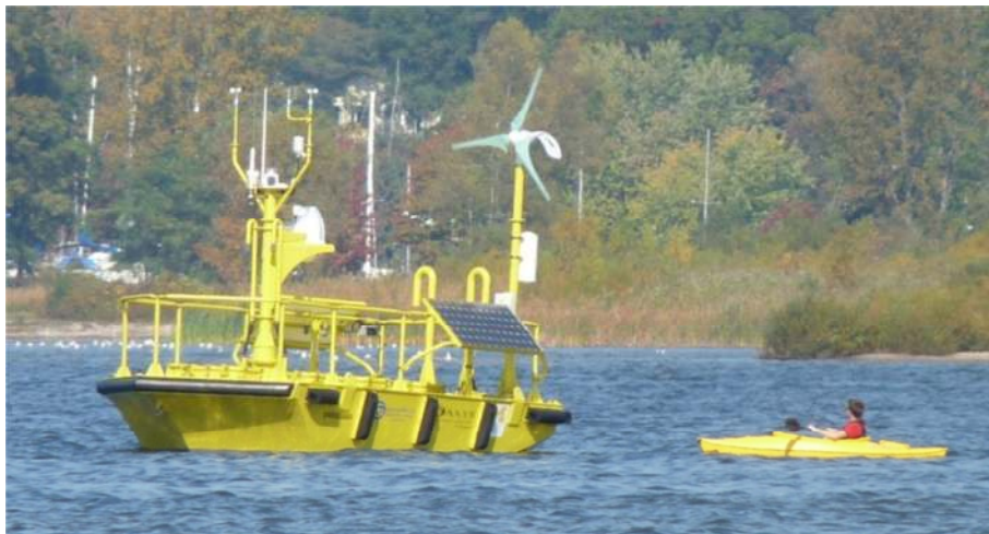
Figure 1: The wind monitoring buoy on site in Muskegon Lake. The egg-shaped device mounted above the deck is the Vindicator laser wind sensor. The kayak offers a sense of scale.
