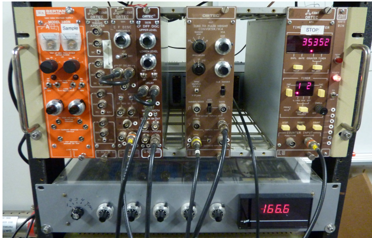
Figure 16: Timing electronics. Starting from top right we have the counter that was used to construct the discriminator curves, the TAC, the stop discriminator, and the start discriminator (the last two modules were not used in our timing electronics).
