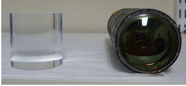
Figure 10: Fast plastic scintillator cylinder and photomultiplier tube.
