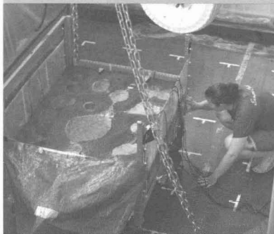
Higgins checks the wetting front during a simulated rainfall
