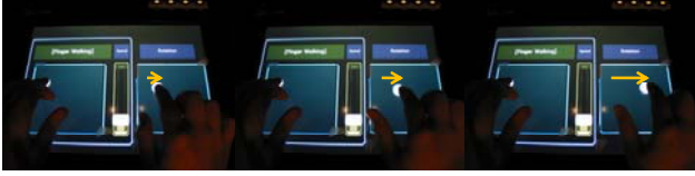
Figure 1. An example of the ‘dragging’ rotation-in-place technique. Dragging from the left to the right means rotating the world clockwise
