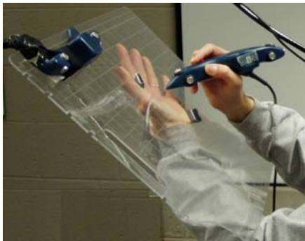
Figure 3: Physical devices used in pen-and-tablet interaction metaphor
