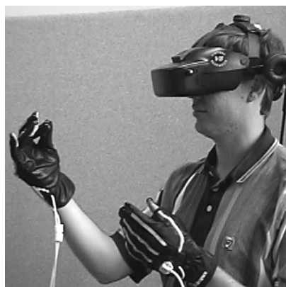
Figure 1. User wearing HMD and Pinch Gloves™
