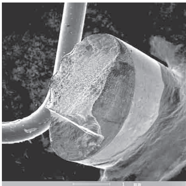
Figure 6 Fracture surface - specimen No. 2
