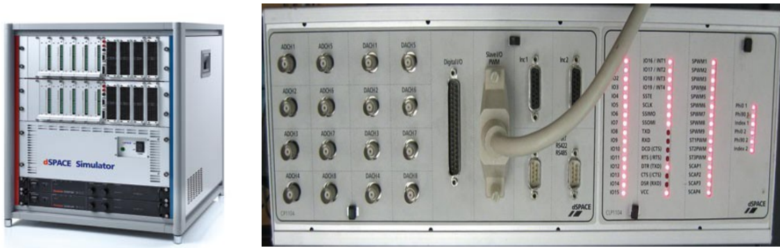
Fig.3.1. The dSPACE simulation and its connector panel [58]
