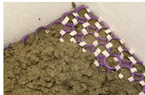
Fig. 5: The example of optical meander in point mode applied in civil engineering.
