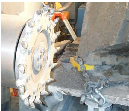
Fig. 1 Interaction between bits and hard rock (i.e. disintegration, experiment)
