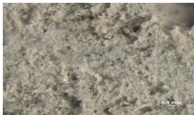
Figure 7 Photograph of building mixes containing polyurethane crumb – mix containing the 1/4 mm polyurethane fraction, magnification 40×
