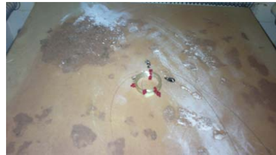
Fig. 11: Detail of disposition of sensory rings n.1 and n.3 inside the high temperature furnace. The photo was taken before the start of the process.
