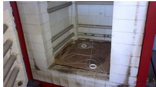
Fig. 7: Placement of sensory rings inside the high temperature furnace. Photo was taken after 45 minutes from the beginning of the process.
