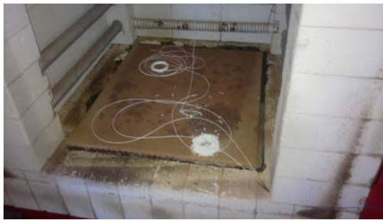
Fig. 10: Shape failure of the sensory ring n.1 from multimode optical fiber with tight secondary protection at a temperature higher than 400 °C.
