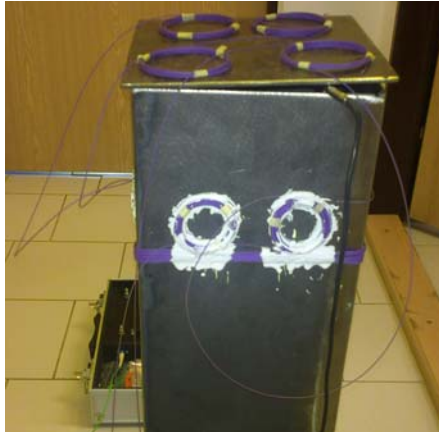
Fig. 21: The crystallizer model with covered upper part and NTC sensor of digital thermometer TESTO 720.
