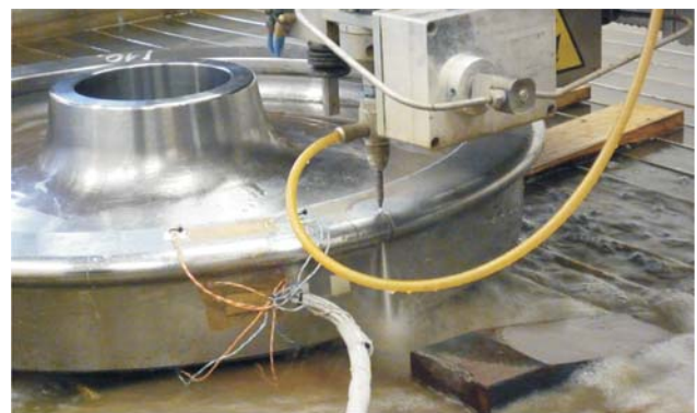
Figure 4 Cutting of railway wheel by abrasive water jet
