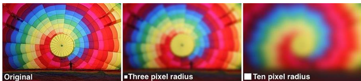
Figure 2.3.4 How different sized kernels affect the Gaussian blur filter, adapted from (Song, 2013) (Creative Commons Attribution).
